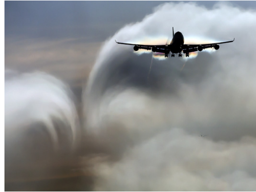
Figure 3. Downwash, trailing vortices and wing region condensation. Korean Air cargo Boeing 747-4B5, at Amsterdam Schiphol, 2013. Copyright Bart Mozer.
