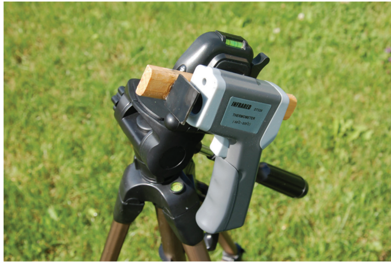
Figure 2. Simple bolometer with infra-red thermometer.
