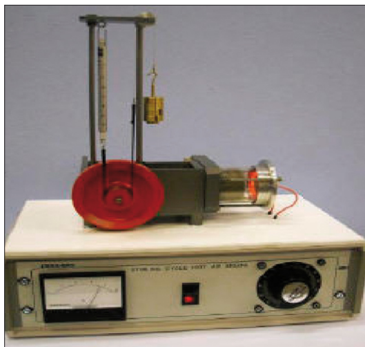
Figure 1. Stirling engine manufactured by Cussons Technology Ltd.
