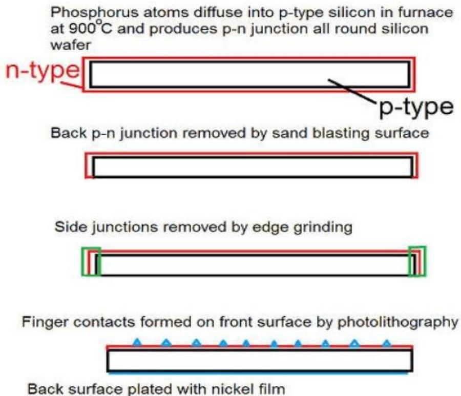
Contacts are then reinforced by giving the complete cell a solder dip.
