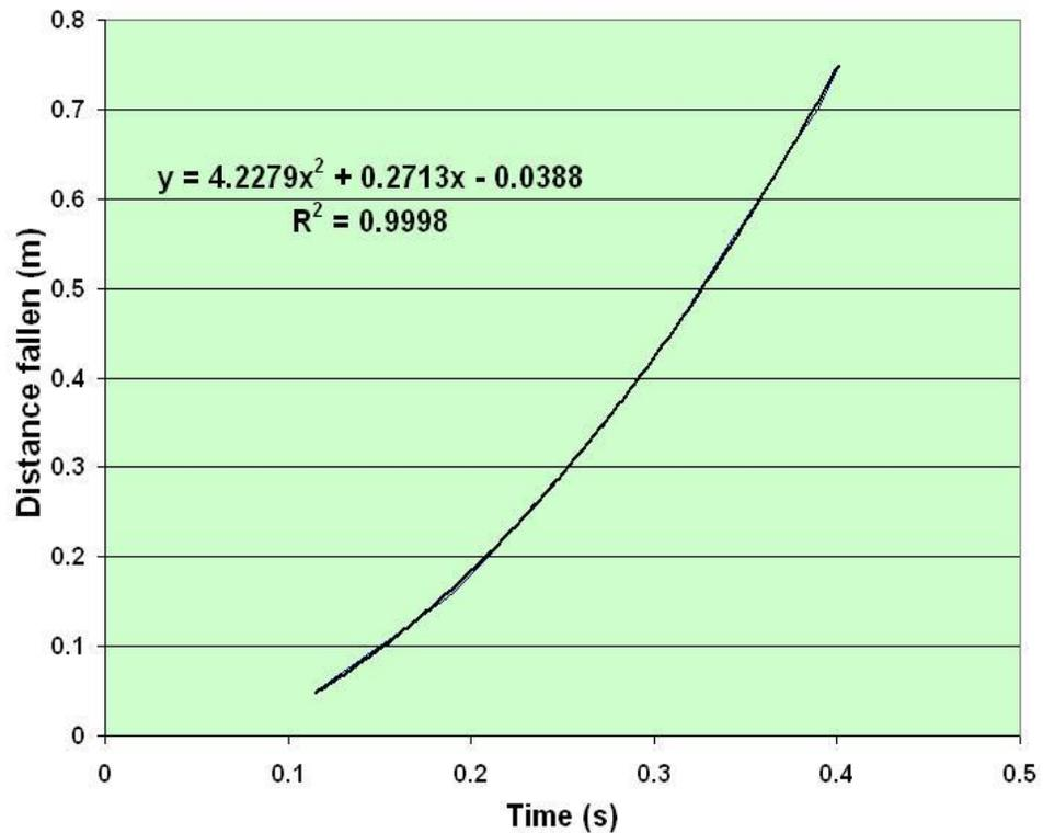
The magnet N\_S poles give rise to positive and negative swings in the induced voltage and, from an EXCEL trace the times of the middle point can be determined. We know that these crossings will occur just when the magnet passes the coil so a time versus "fallen distance" of 0.05 m, 0.10 m, 0.15 m ..... can be plotted. From the laws of motion we have  $s = 0.5 * g * t^2 + u * t$  so the data can be fitted to a polynomial of second order.
