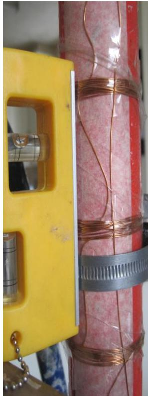
A Picoscope ADC100 is used to record the induced voltage and a "single shot" mode is used. A dc pulse initiated the sweep and this was applied to channel A as a trigger pulse. The signal from the series connected coils were recorded on channel B. Results are presented below and it is clear that these times could never be made with a stop watch. All the peaks occur in a time interval of less than 1/2 second (500 ms).
