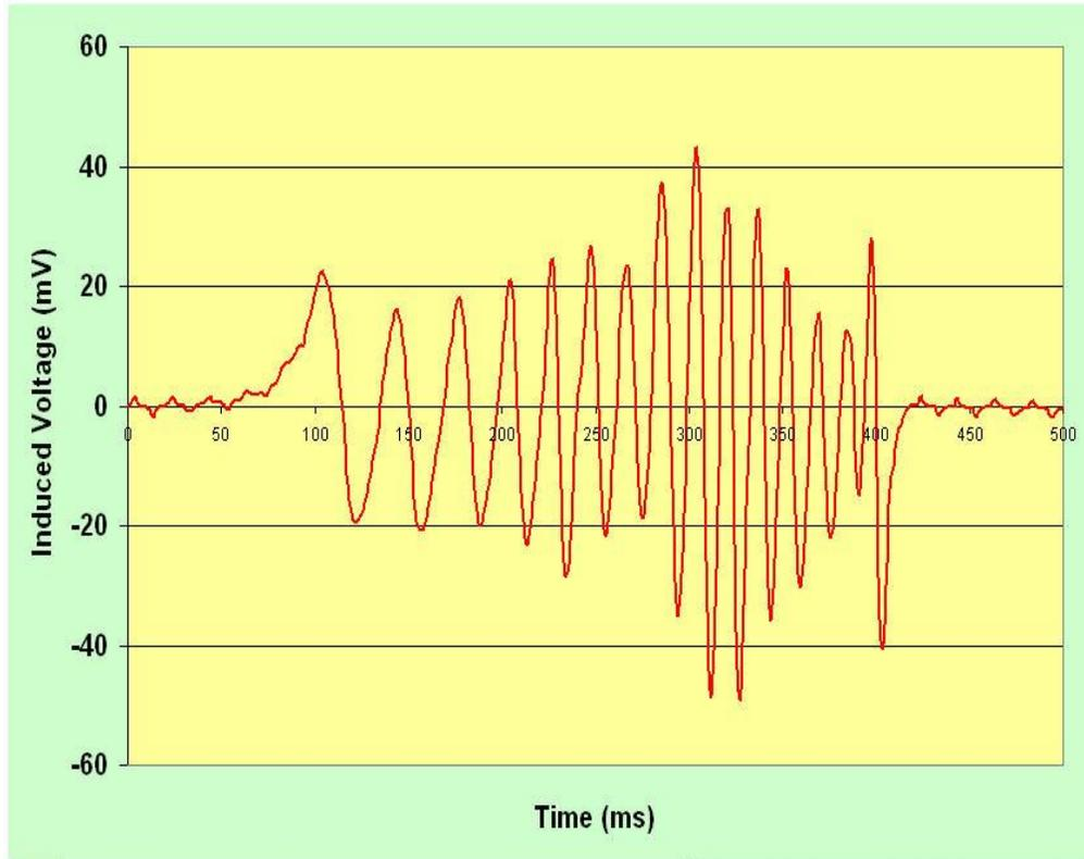
The trace clearly shows that the magnet is moving faster and faster thus confirming that it is acted on by the gravitational force. The envelope of the trace cannot be explained though it may be due to the fact that the trajectory of the magnet is not precisely on the center-line of the tube
