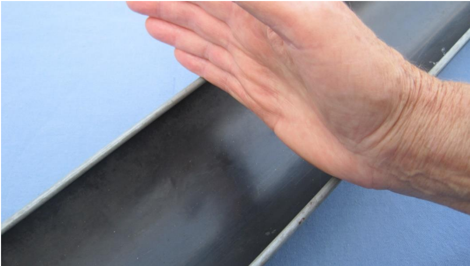
Fig 9 Identifying nodes and anti-nodes of standing wave modes on Lecher Lines (hands-on approach)
