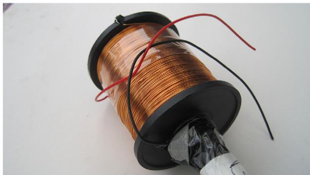
**Figure 1.** Bobbin of enamelled copper wire (outer diameter of wire is 0.37 mm) used as a magnetic field sensor. The handle can be made of a wood or plastic rod.
