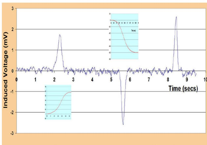
**Figure 2.** Induced voltage produced from a 180° flip of the bobbin in the Earth's magnetic field, integration profiles are inserted for two of the peaks (see appendix).
